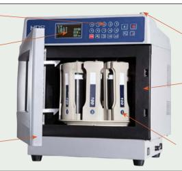
Push-type open-door button at the top, easy & reliable in operation.
