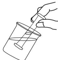
(3) Immerse the tube in the sample. Release the sides to fill the tube up to the half. Shake the tube lightly 5-6 times.
