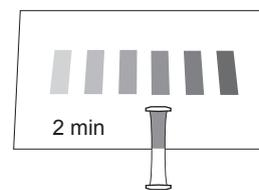
(4) After 2 minutes, put the tube on the color chart as shown and compare with the standard colors.
