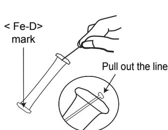
(1) Remove the line to clear the aperture from the top of the tube.
